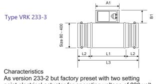
As version 233-2 but factory preset with two setting point electrical actuator for operating voltage of 230 volt. Type 233-4 as 233-3 but with additional auxiliary switch for an additional setting command.
